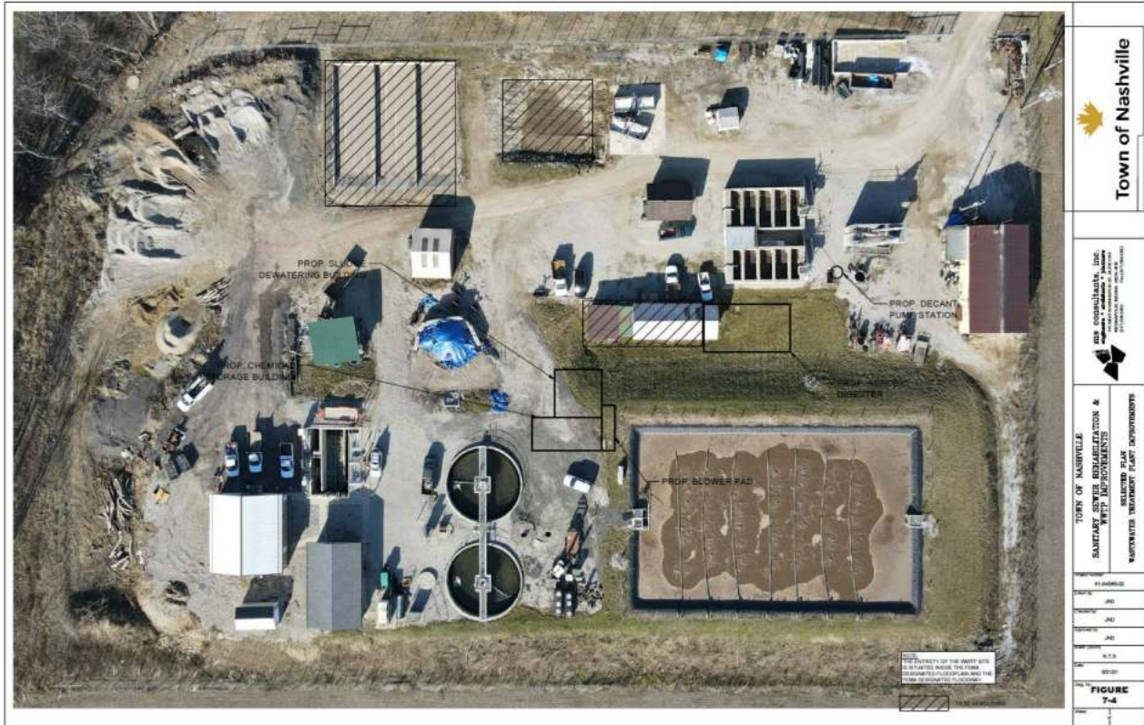
Figure 7-4- Selected Plan: WWTP Sludge Improvements
